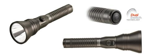
Material/Lens 6000 series machined aircraft aluminum with anodized finish. Unbreakable polycarbonate lens with scratch-resistant coating. O-ring sealed.
