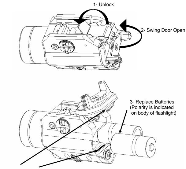
4- Insert Tab into Slot to Close Door
